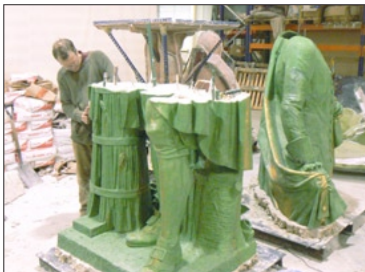
Fine detail is added to the waxes from which the final moulds will be made
